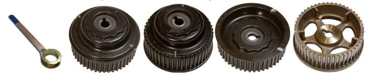
Use AVCS Int Cam Sprocket Tool #501 with these sprockets
